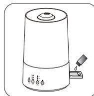
Add 2~3 drops of essential oil on the fragrance cushion. Plug in the power cord and turn on the switch.
